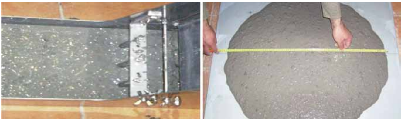
Figure 2. Self-compacting concrete testing by L-box (on the left) and by flow table (on the right)
