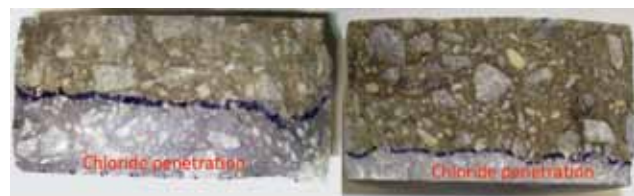
Figure 6. Chloride penetration depth for the mix SCC (left side) and mix SCC-FMP (right side)
