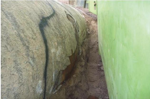
Figure 12. Incipient failure of a 96-inch diameter pipe [57]
