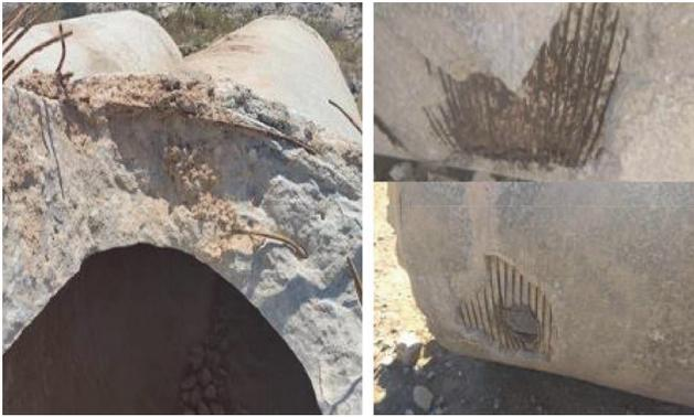
Figure 5. Failed PCCP pipe [6]
