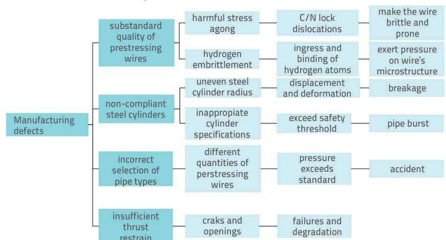
Figure 11. Manufacturing defects in PCCPs
