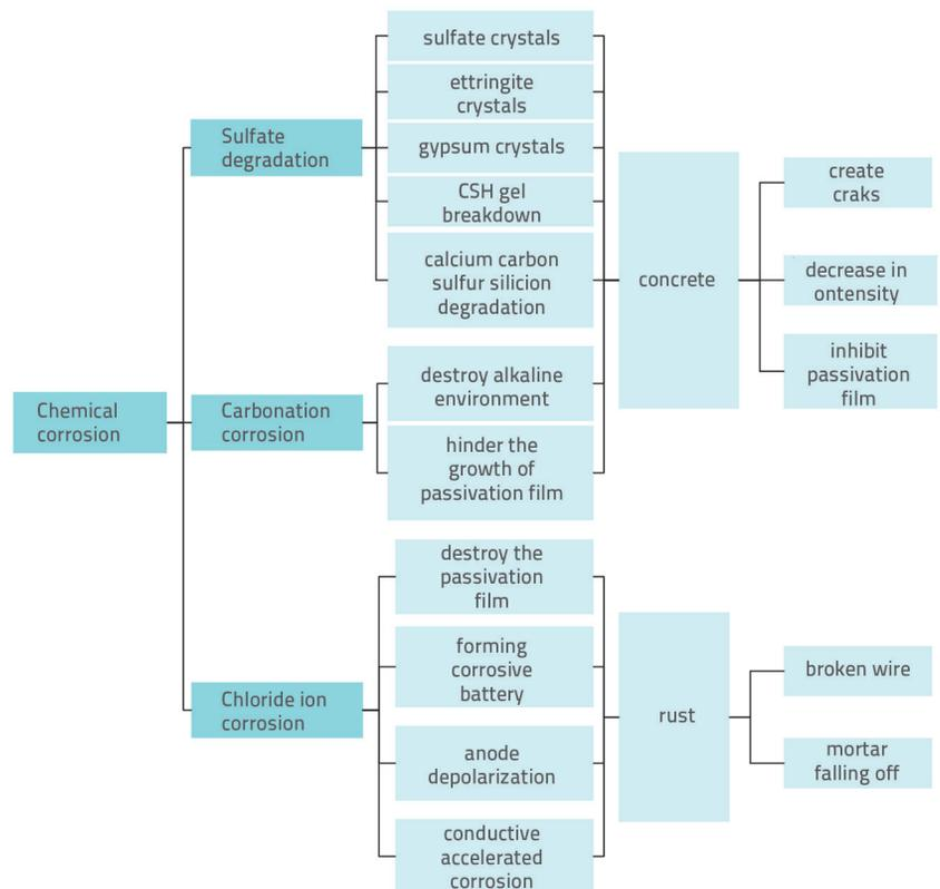
Figure 6. Chemical erosion process of PCCPs
