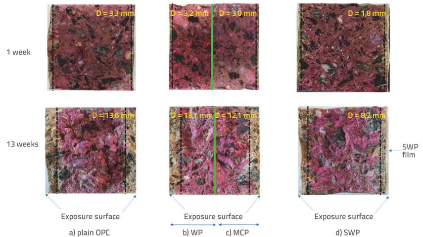
Figure 4. Carbonation depth measurement for: a) plain ordinary Portland cement (OPC); b) WP; c) MCP; d) SWP [30] (Note: Images are not on scale bar)
