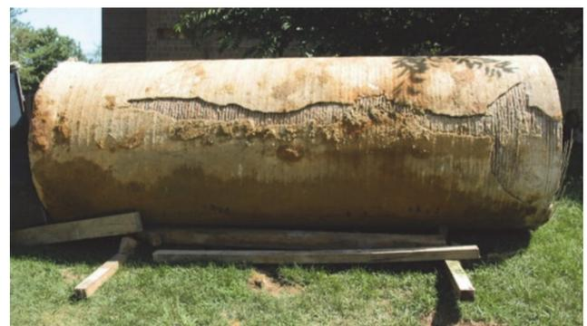
Figure 10. Damaged PCCP [53]
