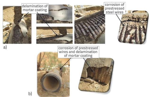
Figure 2. Corrosion of PCCP and prestressed steel wires [7]
