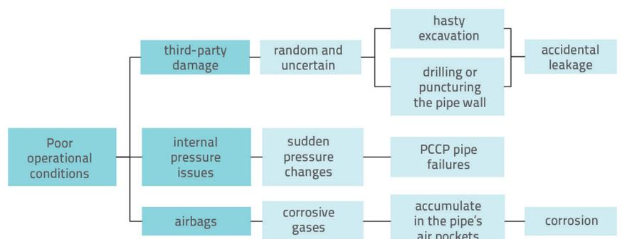
Figure 16. Poor operational conditions of PCCPs
