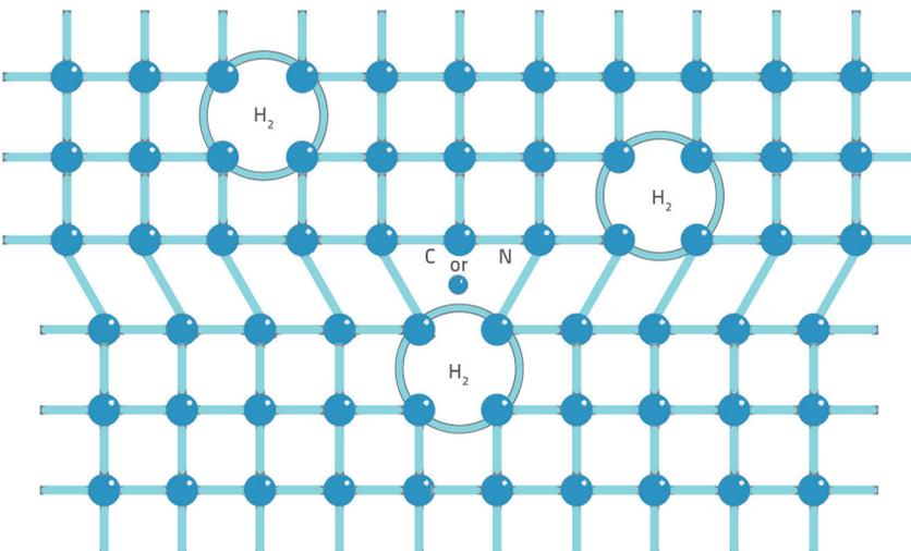
Figure 8. Hydrogen atoms infiltrating a prestressed wire lattice
