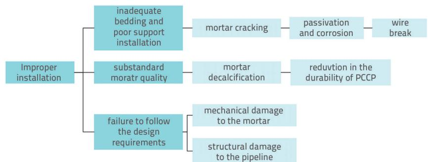
Figure 14. Improper installation of the PCCP
