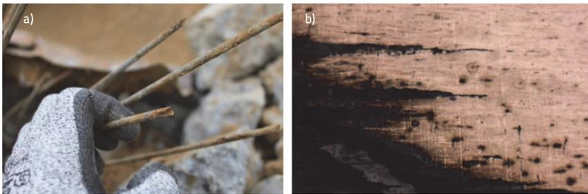
Figure 9. Prestressed wires in field and laboratory [52]: a) Brittle wire fracture surface observed on corroded wires; b) Longitudinal splits and corrosion oriented along the wire axis
