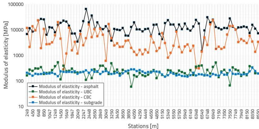
Figure 12. D28 pavement modulus of elasticity D28 [37]
