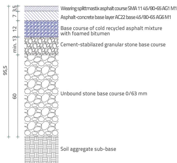
**Figure 14. Layers of strengthened pavement structure of D28 Bjelovar bypass state road [35]**
