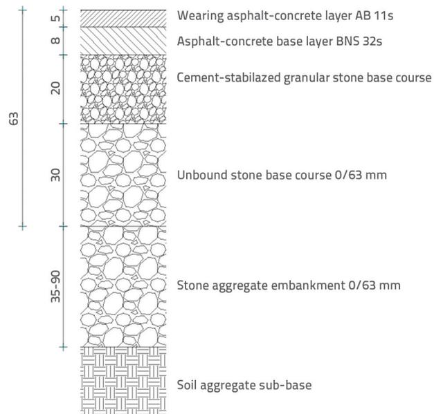
Figure 13. Layers of the existing state road structure D28 [35]
