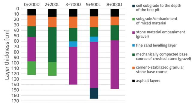
Figure 7. Graph of layer thickness and composition of pavement structure [38]
