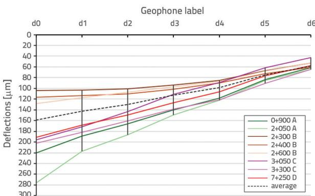
Figure 10. Values of pronounced high and low deflections in analyzed subsections (A, B, C and D)
