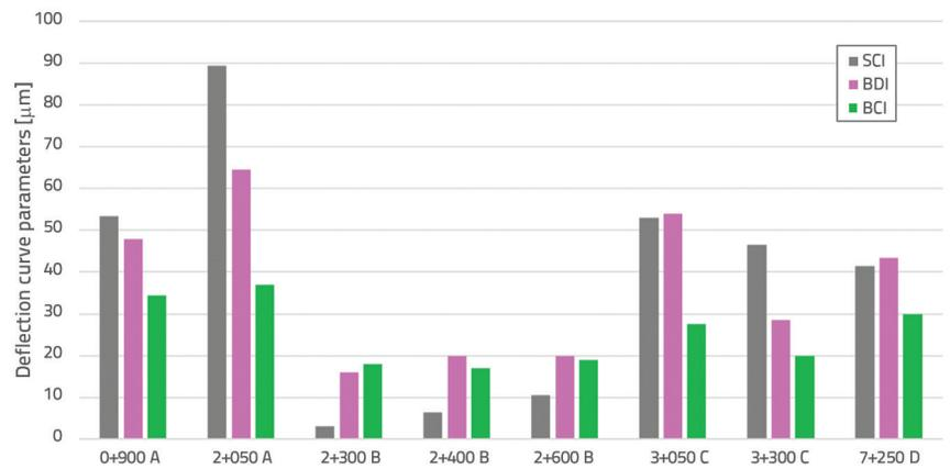
Figure 11. Deflection curve parameters with low and high deflections in analyzed subsections (A, B, C and D)
