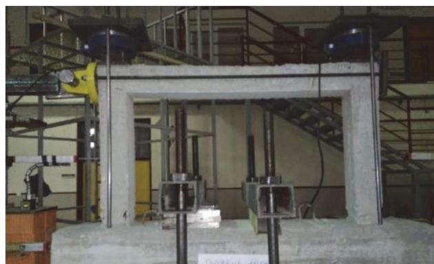
Figure 7. Cyclic test of the bare frame
