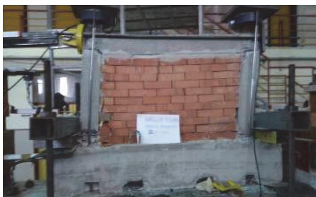
Figure 18. Frame with dry-stack masonry infill and mortar joint with a large displacement of 80 mm (drift ratio of 0.1)
