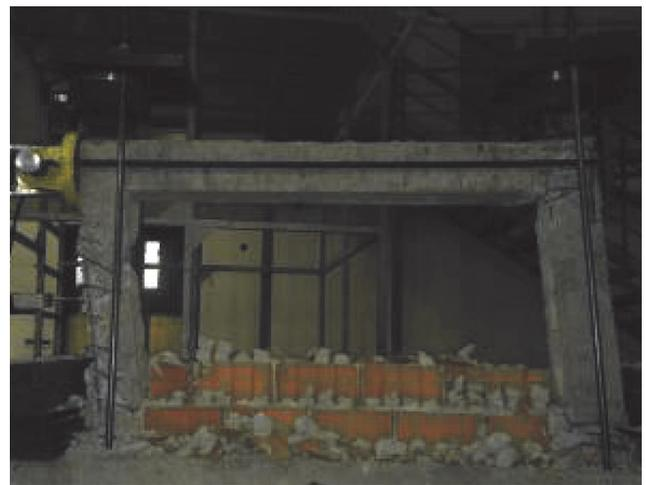
Figure 21. Damaged frame with conventional infill at the maximum displacement (drift ratio of 0.08)
