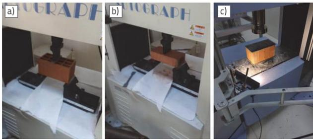
Figure 5. a) Bending test of the hollow brick specimen; b) Bending test of the clay brick specimen; c) Compression test of the hollow clay brick
