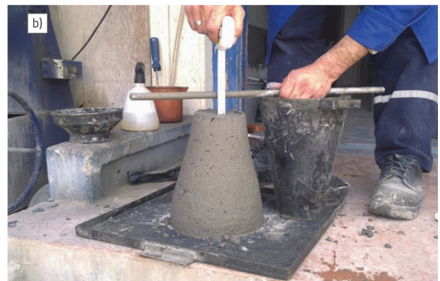
Figure 4. a) Compressive strength values of a set of cylindrical samples obtained from the T5 mixture; b) Slump cone test of the T5 mix design showing the 4 cm slump
