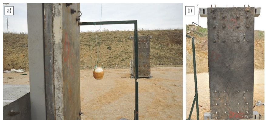
Figure 18. a) C4 blast placed 25 cm away from the face of the panels; b) Panel face after the explosion showing blast burns but no observable structural damage
