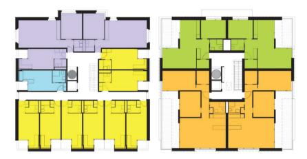
Figure 5. Typical (left) and attic (right) floor plans (1-room, 2-room, wheelchair-accessible apartments, 2.5-room, -3.5-room -ventilation shaft). Photo credit: Kämpfen für Architektur [24]
