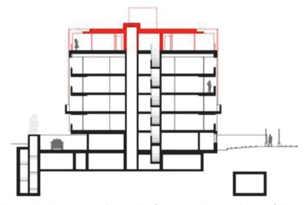
Figure 4. Vertical intersection of the building (floor added during retrofitting, red), Photo credit: Kämpfen für Architektur [24]
