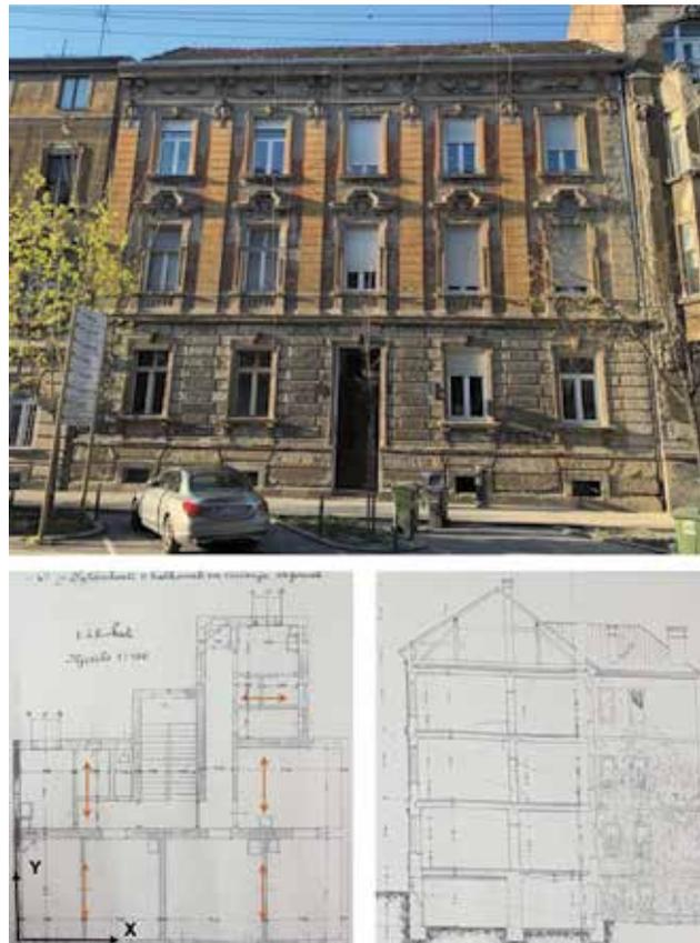
Figure 3. Copy of original floor plan and cross-section of the building (bottom), photograph of the building (top)
