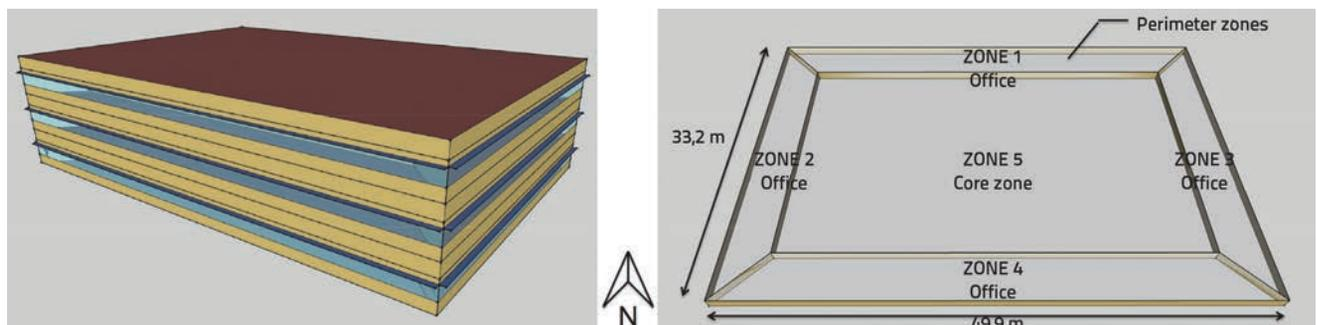
Figure 2. Overall geometry and floor plan showing thermal zones of the base-case office building
