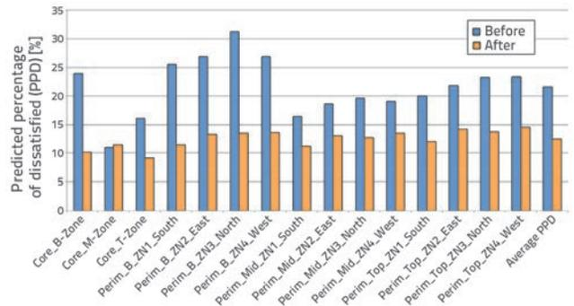
Figure 4. PPD values of building zones before and after energy efficiency improvement at building envelope
