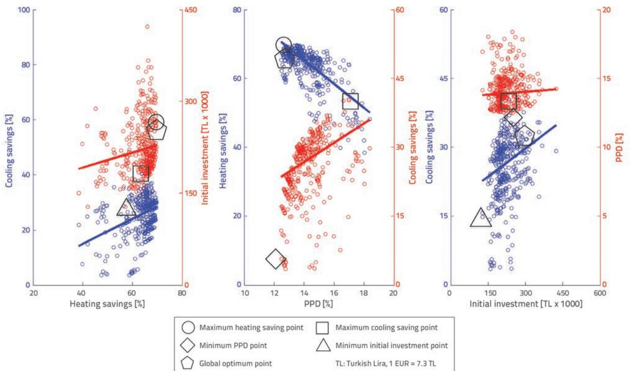
Figure 3. Multi-objective optimization results including pairwise relationships and trends: Heating Energy Saving, Cooling Energy Saving, PPD and Initial Investment. The graphs are plotted on dual Y-axes with blue data points belonging to the left axis, and red ones to the right axis
