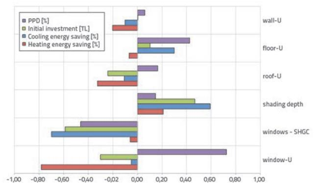
Figure 5. SRC sensitivity indices of input parameters for heating energy savings, cooling energy savings, PPD and initial investment
