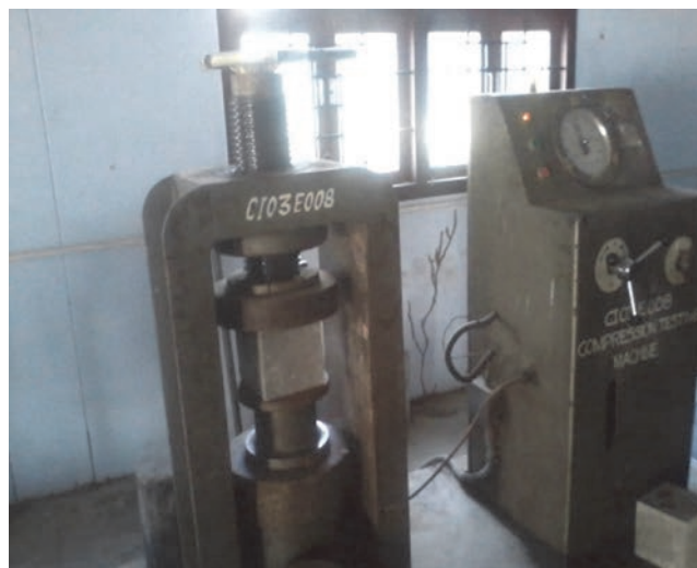
Figure 12. Compressive strength test on oven dried cubes
