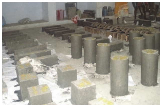
Figure 3. Specimen casting in progress
